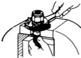
**V** Screw the collar onto the fitting by hand to begin with, and then, with the fitting mounted in the vice, with the correct-sized spanner. It is not necessary to screw the collar on all the way (although this is acceptable) – a gap of about 0.025 – 0.040" (0.65 – 1.00mm) between the collar and the fitting is generally desirable. If assembling angled fittings or banjo fittings, check the alignment of the hose ends before turning the final turn.
